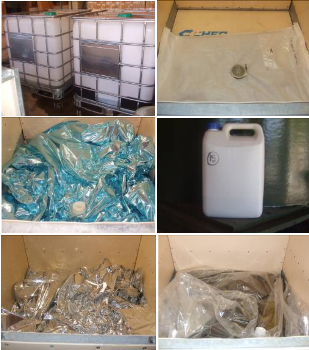
Figure 3.2 Examples of the range of plastic containers being tested including Ecobulk tank, metallised bags, 4 litre bottle
