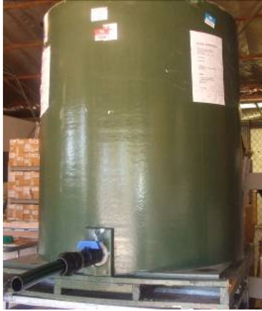
Figure 3.1. Original cylinder containing a metallic lined collapsible bag with 1000 L extra virgin olive oil. A polythene pipe connector was used to dispense the oil.
